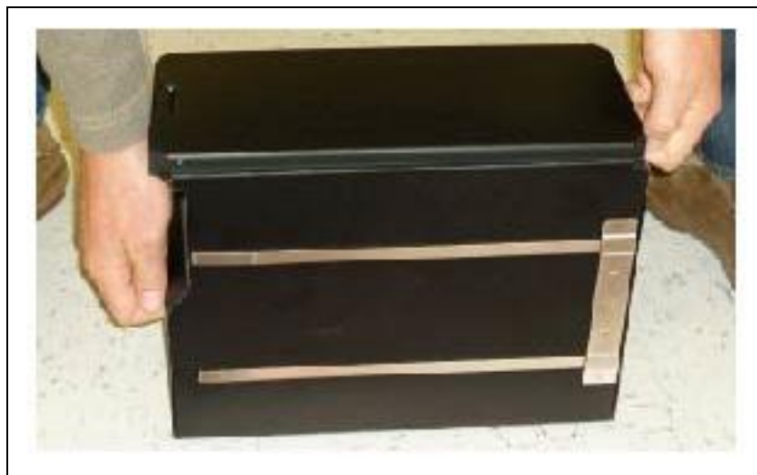
Figure 3-10 Correct Way to Lift the Battery
