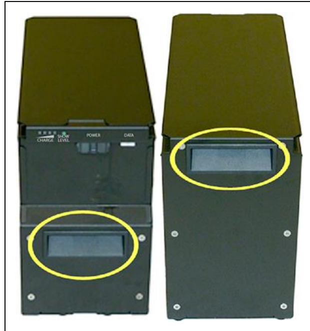
Figure 3-9 Recessed Handles for Lifting the Battery.
