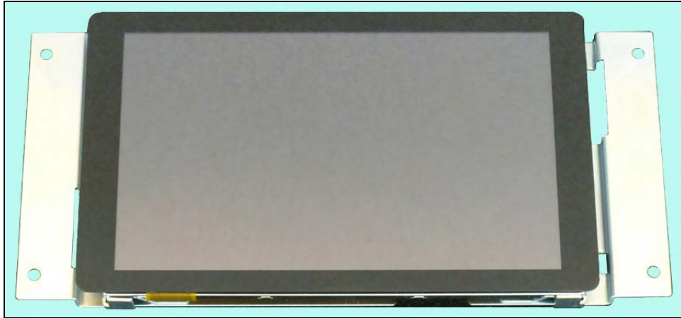
Figure 4-2. Front of Touchscreen with Bracket
