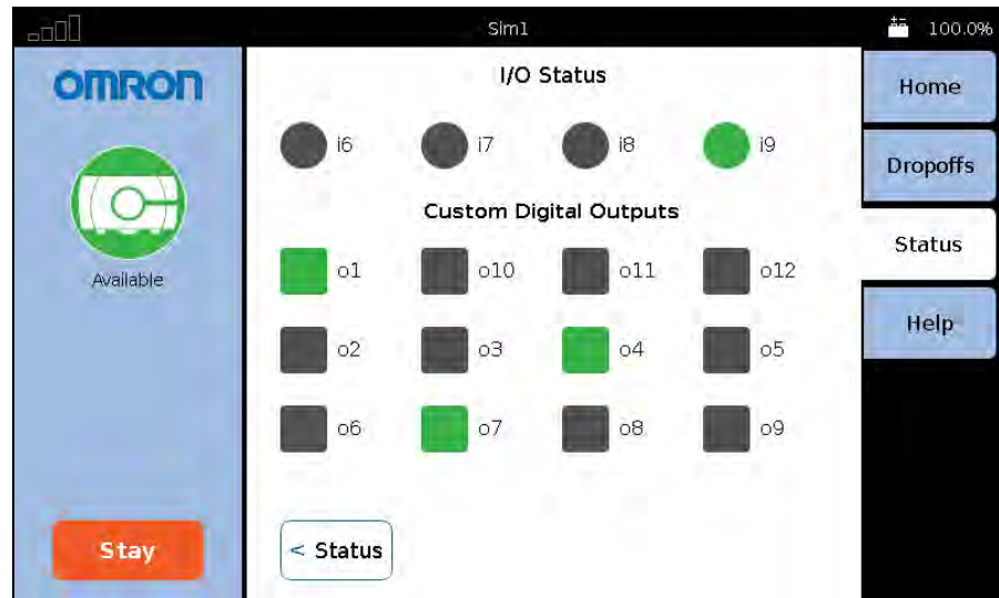
Figure 4-15. Status > I/O Screen (Top Inputs are not shown in this example)
