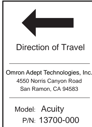
Figure 6-5. Label on Camera Mounting Bracket
