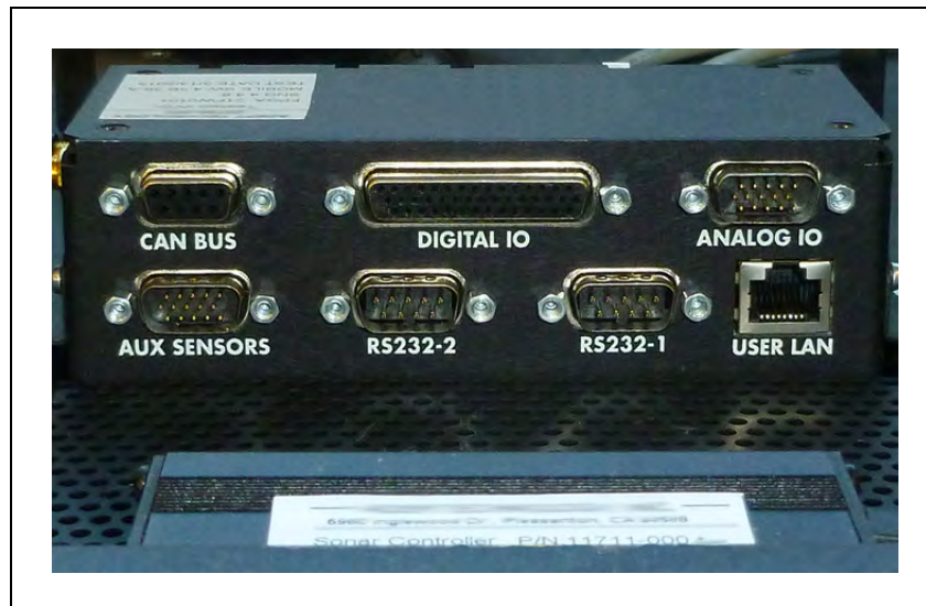
Figure 8-9. Upper Front of Core, Showing RS232 Ports
