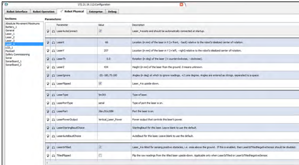
Figure 7-2. MobilePlanner Side Laser Parameters
