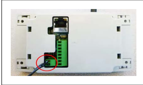
Figure 5-19. VDC Connection on Back of Box Body (Circled)
