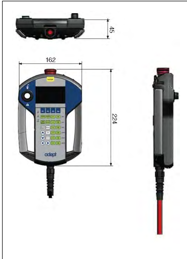
Figure 5-3. T20 Pendant Dimensions (Units in mm)
