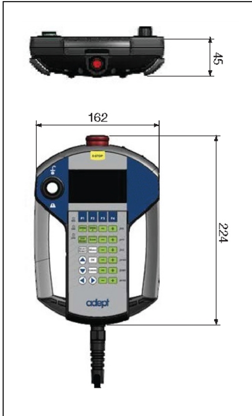
Figure 6-1. T20 Pendant Dimensions (Units in mm)
