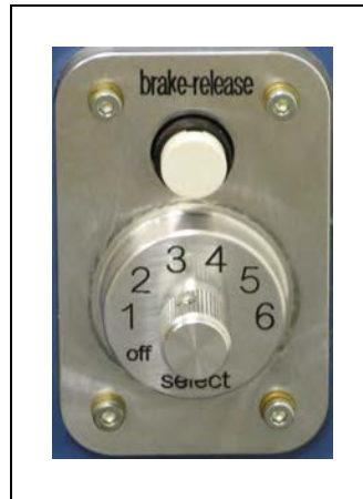
Figure 6-2. Brake Release Switch on UL Robots
