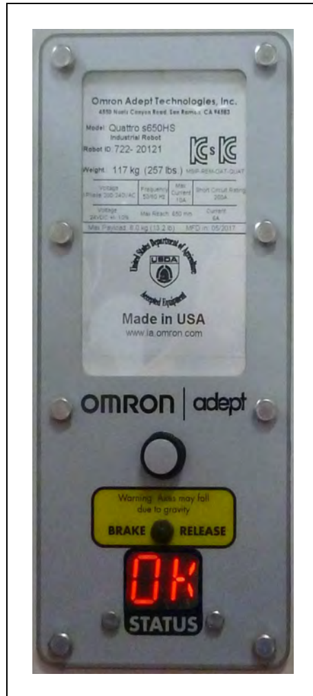
Figure 10-8. Status Display Panel, Showing 8 Hex-head Bolts
