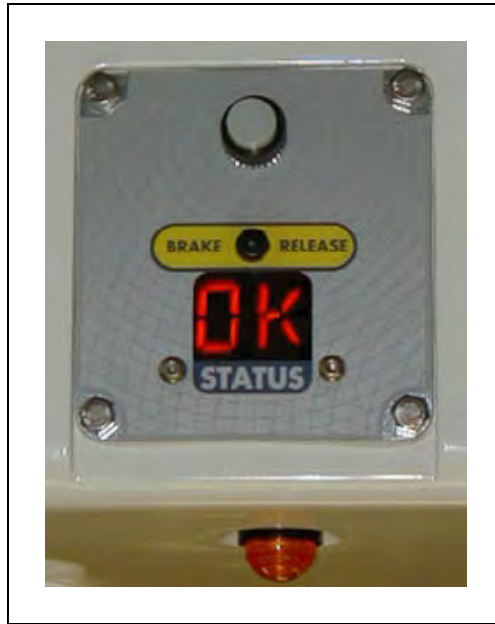
Figure 9-10. Status Display Panel, Showing 4 hex-head Bolts
