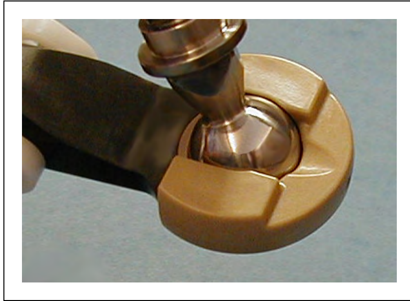
Figure 7-2. Ball Stud Lock on Ball Joint Socket
