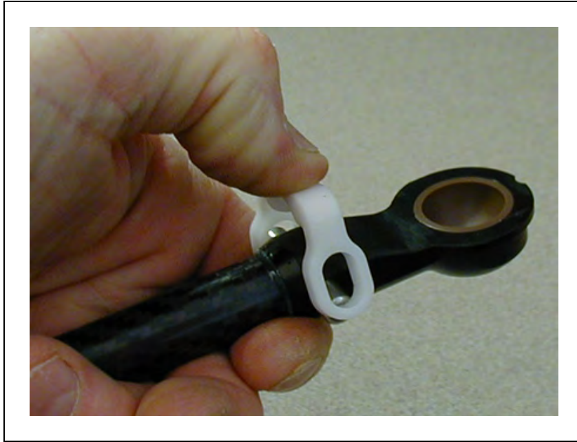
Figure 10-15. Squeezing the Horseshoe into Position, H Shown
