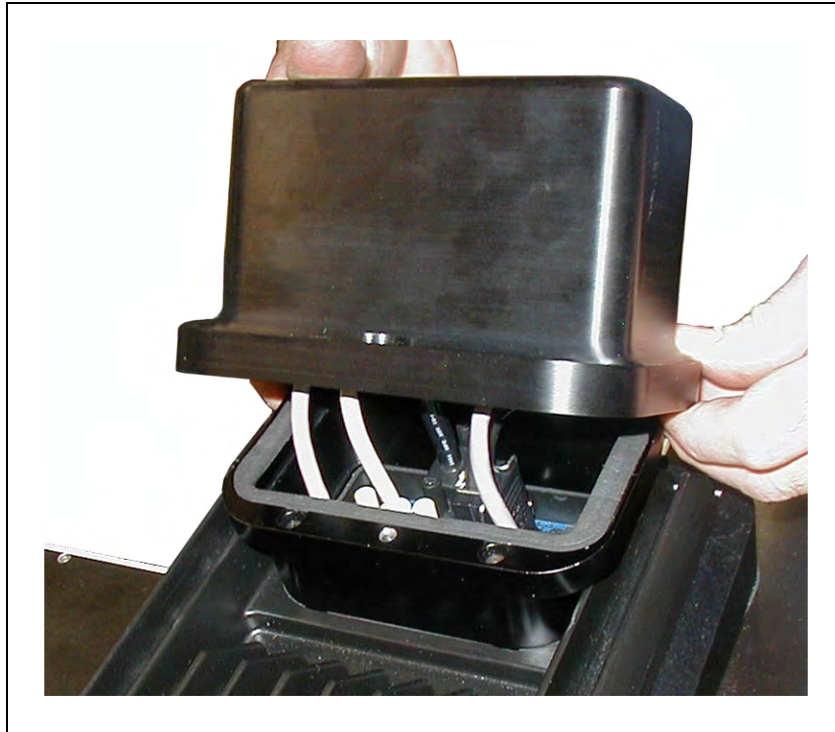
Figure 11-10. Installing Cable Entry Top Cover Assembly
