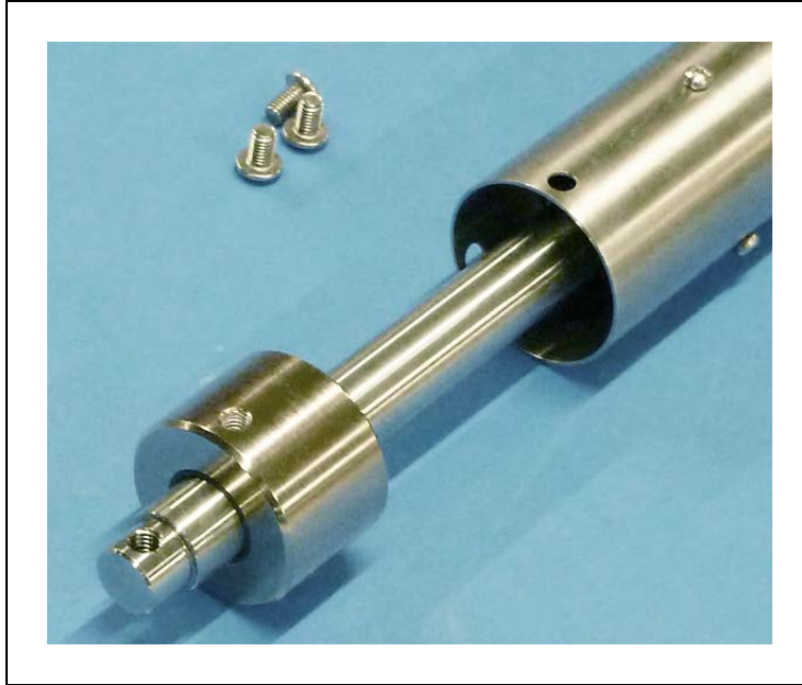
Figure 7-7. End Cap Placed Over Center Shaft
