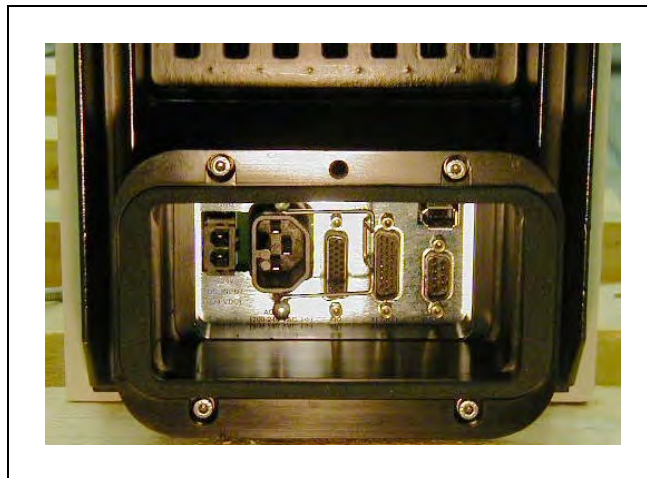
Figure 9-3. Cable Seal Housing Installed
