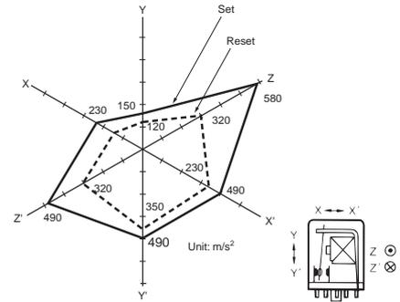
Measurement: Measurement: Shock was applied 3 times each in 6 directions along 3 axes with the Relay set and reset to check the shock values that cause the Relay to malfunction.
