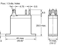
Mounting Holes (BOTTOM VIEW) Tolerance: ±0.1 mm
