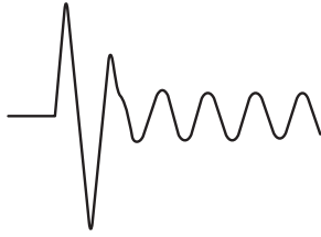
Waveform of Lamp Starting Current
