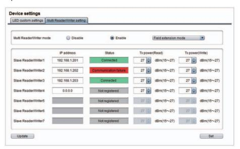
After this, the multiple Reader/Writers shall jointly operate by the issuing of communications commands from the host device to the master Reader/Writer.
