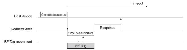
If RF Tag exist in the communications range and communications with the RF Tag fails
