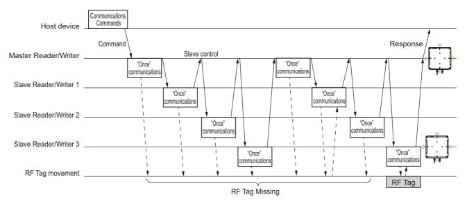
• If the RF Tag completes normally in any of the Reader/Writers in multiaccess
