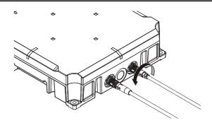
Hold onto the connector on the Power Cable and pull it straight out to remove it.
