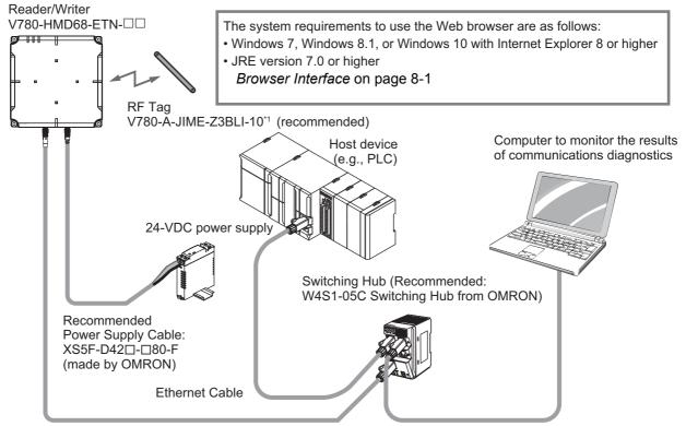
Recommended Ethernet Cable: XS5W-T42□-□ME-K (made by OMRON) \*1. This is the model number for one package of 10 RF Tags. Order the number of packages that you require.
