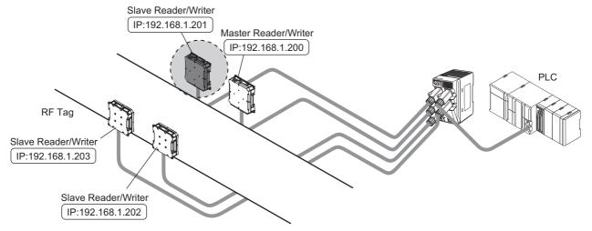
After the slave Reader/Writer communications processing has completed one cycle, operation will repeat from Procedure 2.
