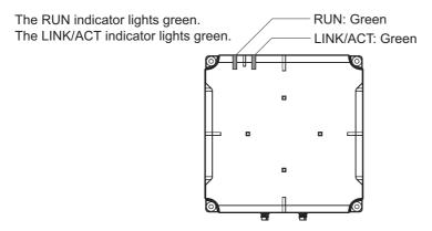
The RUN indicator will flash at 0.4-s intervals when the Reader/Writer starts in Safe Mode.
