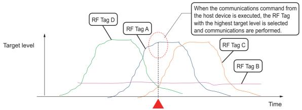
· One or More RF Tags in the Communications Range After the Reader/Writer selects an RF Tag in the communications range, it returns the response without waiting for a timeout.
