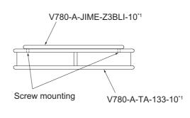
**2** Mount the Attachment to which the RF Tag is mounted to the metallic material. Mount it with two M4 bolts.
