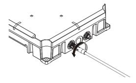
Hold onto the connector on the Ethernet Cable and pull it straight out to remove it.
