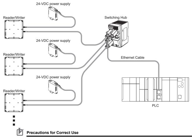
To connect more than one Reader/Writer, all devices must be set to a unique IP address.
