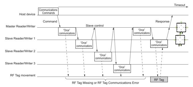
If communications with an RF Tag completes abnormally in any of the Reader/Writers in single-access
