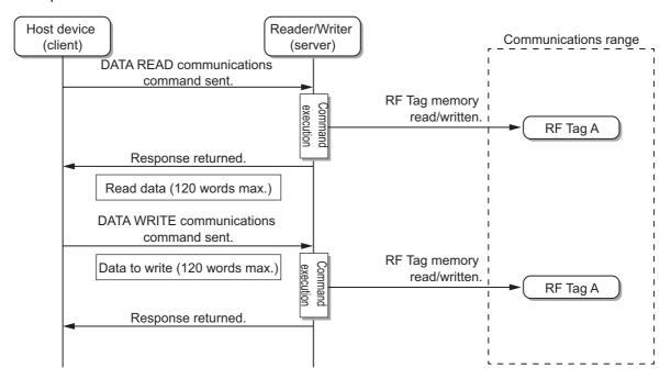
If communications with an RF Tag are not possible, a "failure in slave device" exception code (04 hex) is returned in an error response. Following the error response reception procedure.
