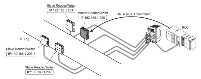
The master Reader/Writer will communicate with the RF Tags with the "Once" communications option. Here, if the communications have ended normally, or if the communications have ended with an error, a response is returned to the host device, and the processing ends. If an RF Tag Missing error or a communications error is detected, it will progress to step 3.
