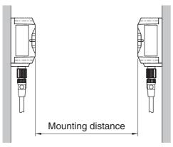
• Installing the Reader/Writer in Parallel
