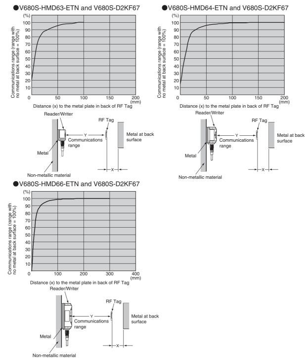
If you use more than one RF Tag, separate them by at least the interval shown below to prevent malfunctions due to mutual interference.
