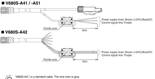
V680S-A4□ is a standard cable. The wire color is gray. V680S-A5□ is a robot instrumentation cable. The wire color is black.
