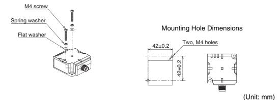
When you install the Reader/Writer, prepare the metal plate shown in the following figure. When the metal plates size is larger than the below illustration, communication range will change.
