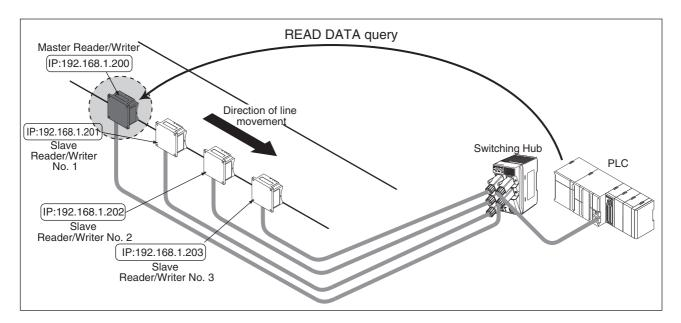
2. The Master Reader/Writer will wait for an RF Tag to enter the communications field and then communicate with the RF Tag. Here, if an RF Tag communications error occurs, the Reader/Writer will return a response to the host device, and processing will end. If communications with the RF Tag end normally, processing returns to step 3.
