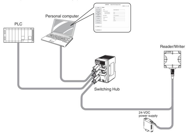
You can connect a computer to the Switching Hub to easily set up the Reader/Writers and check the status of the Reader/Writers.
