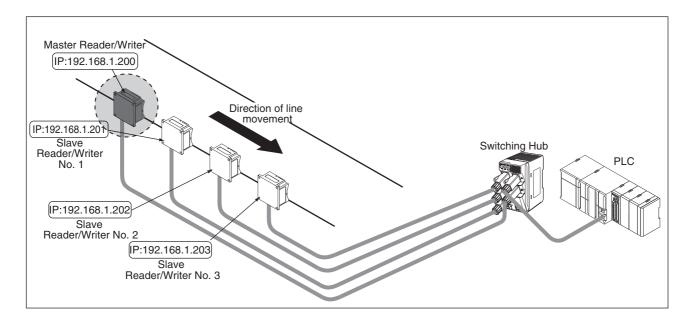
**3.** Slave No. 1 will wait for an RF Tag to enter the communications field and then communicate with the RF Tag. Here, if an RF Tag communications error occurs, the Reader/Writer will return a response to the host device, and processing will end. If communicating with the RF Tag ends normally, processing will be continued in order by Slave No. 2 and then by Slave No. 3.
