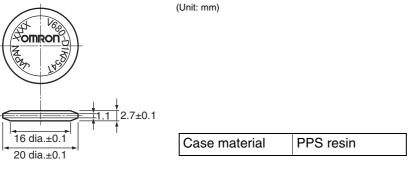
The V680-D1KP54T RF Tag can be placed in the Attachment in either direction. The direction does not affect operation.
