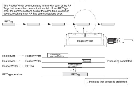
FIFO Trigger communications cannot be used for communicating with V680-D1KP  $\Box \Box$  RF Tags.
