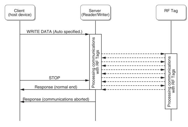
Example: Processing was aborted when a STOP query was received immediately after completing processing after the Reader/Writer detected an RF Tag.
