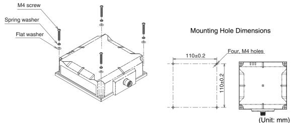
When you install the Reader/Writer, prepare the metal plate shown in the following figure. When the metal plates size is larger than the below illustration, communication range will change.
