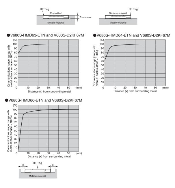
If you use more than one RF Tag, separate them by at least the interval shown below to prevent malfunctions due to mutual interference.
