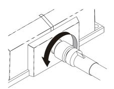
**2.** Hold the base of the Cable connector and pull it straight out.
