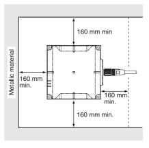
Do not bend the cable into a curve tighter than 40 mm in radius.
