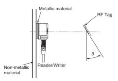
V680S-HMD66-ETN and V680S-D2KF67M (Metal at Back Surface: Steel)
