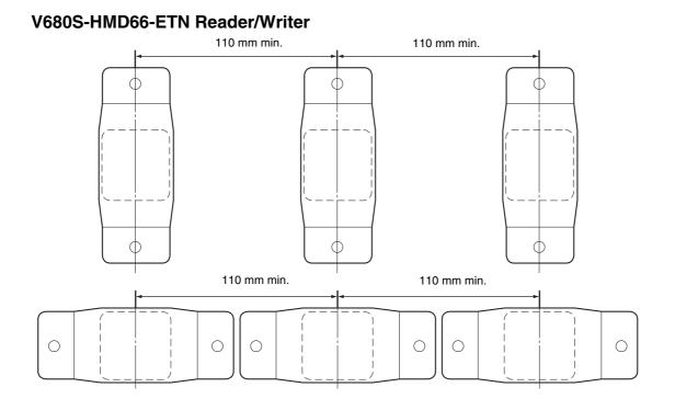
Install the Reader/Writer and RF Tags so that the Reader/Writer and RF Tags are as parallel to each other as possible.
