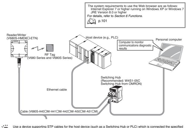
Use a device supporting STP cables for the host device (such as a Switching Hub or PLC) which is connected the specified Cables (V680S-A41  $\Box$ M/-A42  $\Box$ M/-A51  $\Box$ M). Ground the host device to a ground resistance of 100  $\Omega$  or less. CHECK!
