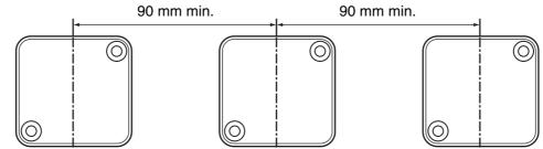
Install the Reader/Writer and RF Tags so that the Reader/Writer and RF Tags are as parallel to each other as possible.
