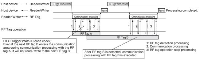
\* When using FIFO Trigger (With ID code check), the ID code of the RF tag is checked. Even if the next RF tag enters the communication area during "communication processing" with the detected RF tag, there is no possibility of reading / writing the next RF tag. However, compared with "Without ID code check", communication time will be longer.
