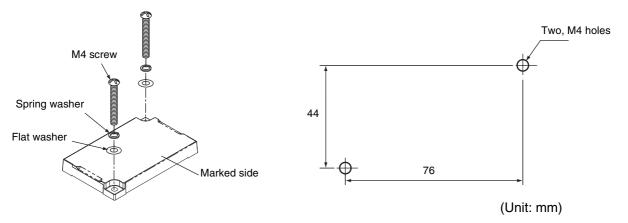
Refer to *RF Tag Installation Precautions* in *Section 11 Appendices* for information on the effect of metal at the back surface, Mutual Interference of RF Tags and Influence of Inclination of the V680S-D2KF68. f = 1, 285
