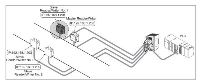
**4.** If an RF Tag missing error is detected for Slave No. 3, the error is returned to the host device and processing ends.
