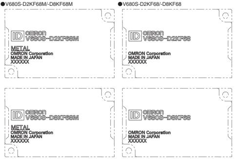
The marked surface is the communications surface. When mounting the RF Tag, face the marked surface toward the Reader/Writer.
