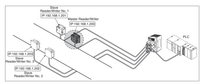
**3.** Slave Reader/Writer No. 1 will communicate with the RF Tag using the Once communications option. Here, communications will end normally or an RF Tag communications error will occur, the Reader/ Writer will return a response to the host device, and processing will end. If an RF Tag tag missing error is detected, processing will be continued in order by Slave No. 2 and then by Slave No. 3.
