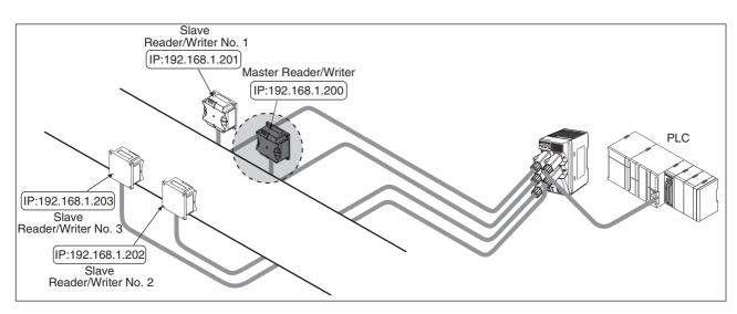
**3.** Slave Reader/Writer No. 1 will communicate with the RF Tag using the Once communications option. Here, communications will end normally or an RF Tag communications error will occur, the Reader/ Writer will return a response to the host device, and processing will end. If an RF Tag tag missing error is detected, processing will be continued in order by Slave No. 2 and then by Slave No. 3.
