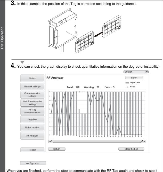
When you are finished, perform the step to communicate with the RF Tag again and check to see if stable communications have been achieved.
