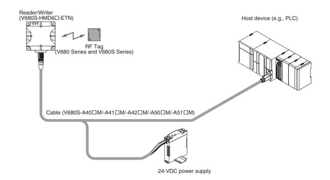
Use a device supporting STP cables for the host device (such as a Switching Hub or PLC) which is connected the specified Cables (V680S-A41  $\square$ M/-A42  $\square$ M/-A51  $\square$ M). Ground the host device to a ground resistance of 100  $\Omega$  or less.
