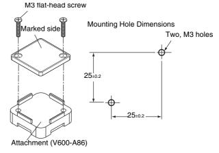
Refer to *RF Tag Installation Precautions* in *Section 11 Appendices* for information on the effect of metal at the back surface, Mutual Interference of RF Tags and Influence of Inclination of the V680-D1KP66T.  $f(\Xi)$  *p.285*
