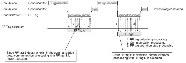
\* When using FIFO Trigger (Without ID code check), the ID code of the RF tag is not checked. Therefore communication time will be shorter than FIFO Trigger (With ID code check). However, if the next RF tag enters the communication area during "communication processing" with the detected RF tag, there is a possibility of reading / writing the next RF tag.
