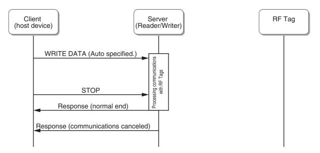
Example: Processing was aborted when a STOP query was received after the Reader/Writer detected an RF Tag but before it completed processing.
