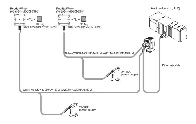
Use a device supporting STP cables for the host device (such as a Switching Hub or PLC) which is connected the specified Cables (V680S-A41  $\Box$ M/-A42  $\Box$ M/-A51  $\Box$ M). Ground the host device to a ground resistance of 100  $\Omega$  or less. CHECK!
