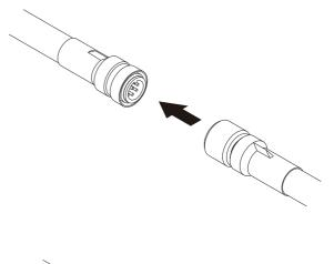
2. Turn the connector on the V680S-A41□M/-A51□M Cable clockwise to lock it in place. Recommended tightening torque: 0.39 to 0.49 N·m
