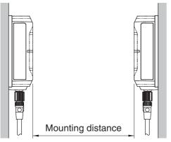
Reader/Writers Installed in Parallel
