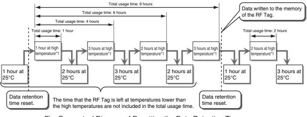
Fig. Conceptual Diagram of Resetting the Data Retention Time
