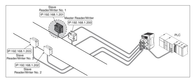
**4.** If an RF Tag missing error is detected for Slave No. 3, communications processing is returned to the Master Reader/Writer and the operation is repeated from step 2.
