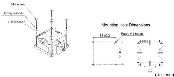
When you install the Reader/Writer, prepare the metal plate shown in the following figure. When the metal plates size is larger than the below illustration, communication range will change.
