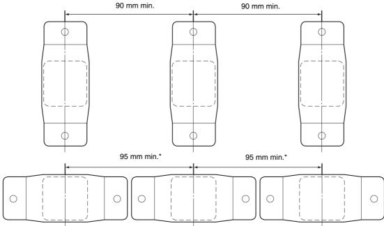
\* This is required for the V680-D1KP66T-SP exterior dimension (Length: 95 mm).
