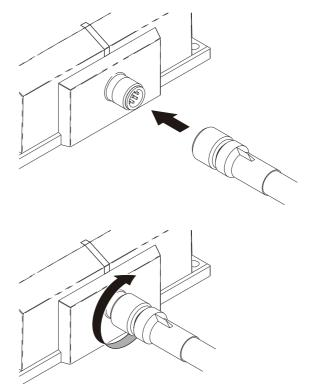
**2.** Turn the Cable connector clockwise to lock Turn the Cable connector clockwise to lock it in place. it in place.
