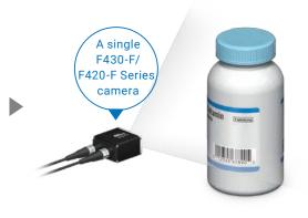
A single camera can now perform both code reading and inspection
