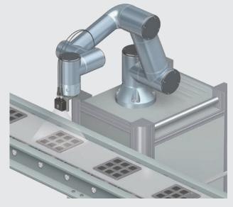
Equipped with a smart camera, the collaborative robot enables simple discriminations that can flexibly handle various objects.
