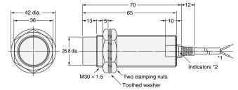
\*1. 6-dia. vinyl-insulated round cable with 2 conductors (Conductor cross section: 0.5 mm2, Insulator diameter: 1.9 mm), Standard length: 2 m 6-dia. vinyl-insulated round cable with 3 conductors
