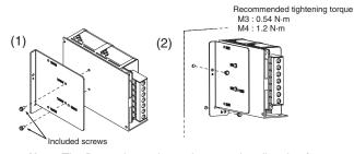
Note: The figure above shows the mounting direction for S82Y-FSG-F32, a similar product. The shape of S82Y-FSG-F31 will be slightly different.
