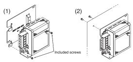
Note: The figure above shows the mounting direction for S82Y-FSG-S22, a similar product. The shape of S82Y-FSG-S23 will be slightly different.
