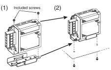
Note: The figure above shows the mounting direction for S82Y-FSG-B01, a similar product. The shape of S82Y-FSG-B03 will be slightly different.
