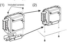
**Note:** The figure above shows the mounting direction for S82Y-FSG-B01, a similar product. The shape of S82Y-FSG-B04 will be slightly different.
