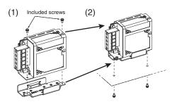
Note: The figure above shows the mounting direction for S82Y-FSG-B01, a similar product. The shape of S82Y-FSG-B05 will be slightly different.
