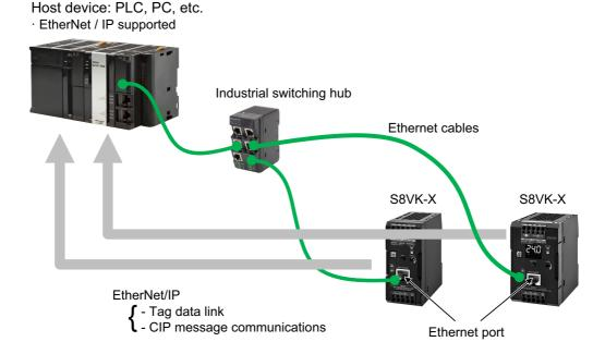
If the S8VK-X was manufactured before February 28, 2019, a tag data link timeout may occur in the network system including the node configured for multicast communications. Use a switching hub with multicast filtering function to prevent multicast packets from reaching S8VK-X.
