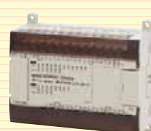
■ CPU Unit with Relay Outputs CPM2A-30CDR-D ■ CPU Units with Transistor Outputs CPM2A-30CDT-D (Sinking) CPM2A-30CDT1-D (Sourcing) 18 input points 12 output points
