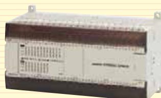
■ CPU Unit with Relay Outputs CPM2A-60CDR-A 36 input points 24 output points
