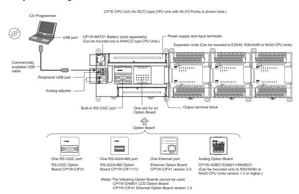
CP1E CPU Unit (An N□□S1-type CPU Unit with 40 I/O Points is shown here.)
