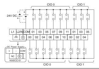
**Input Wiring Diagram**
