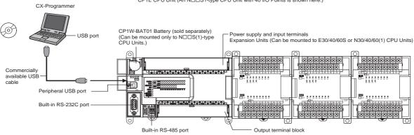
Note CJ1W-CIF11 cannot be connected to the built-in RS-232C port of the CP1E N□□S(1)-type CPU Unit.
