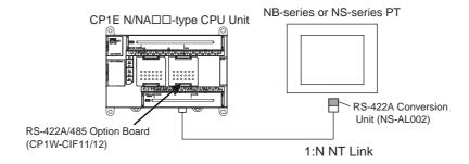
Note Do not use NS-AL002, when connecting the built-in RS-422A port of the NB-series PT.
