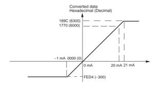
When the resolution is 1/6,000, the 0 to 20 mA range correspond to hexadecimal values 0000 to 1770 (0 to 6,000). The range of data that can be converted is FED4 to 189C hex (-300 to 6,300). A negative current is expressed as a two's complement.
