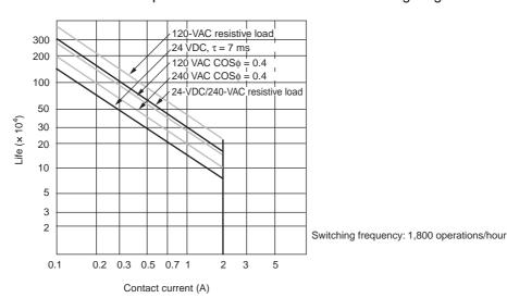
Restrictions of CP1W-16ER/32ER Limit the output load current to satisfy the following derating curve.
