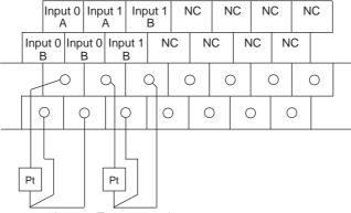
Temperature input 0 Temperature input 1
