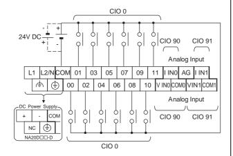
**Input Wiring Diagram**
