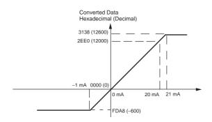
When the resolution is 1/12,000, the 0 to 20 mA range correspond to hexadecimal values 0000 to 2EE0 (0 to 12,000). The entire data range is FDA8 to 3138 hex (-600 to 12,600). A negative voltage is expressed as a two's complement.
