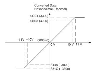
Voltages in the -10 to 10 V range correspond to hexadecimal values F448 to 0BB8 (-3,000 to 3,000). The range of data that can be converted is F31C to 0CE4 hex (-3,300 to 3,300). A negative voltage is expressed as a two's complement.
