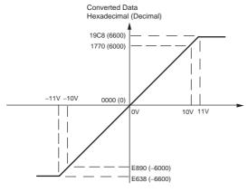
When the resolution is 1/12,000, the -10 to 10 V range correspond to hexadecimal values E890 to 1770 (-6,000 to 6,000). The entire data range is E638 to 19C8 hex (-6,600 to 6,600). A negative voltage is expressed as a two's complement.
