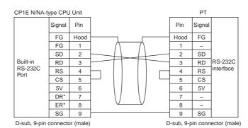
\* DR and ER signals are not supported by the N□□S(1)-type CPU Unit.
