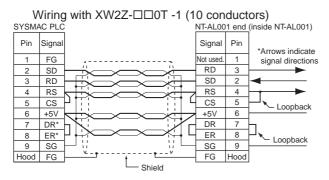
\* DR and ER signals are not supported by the N□□S(1)-type CPU Unit.
