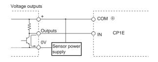
The circuit below should NOT be used for I/O devices having a voltage output.
