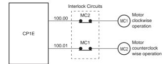
A circuit like the one shown in the diagram on the left is required to prevent outputs MC1 and MC2 from both being ON at the same time even if both PLC outputs CIO 100.00 and CIO 100.01 are both ON.
