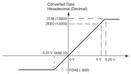
When the resolution is 1/12,000, the 0 to 5 V range correspond to hexadecimal values 0000 to 2EE0 (0 to 12,000). The entire data range is FDA8 to 3138 hex (-600 to 12,600). A negative voltage is expressed as a two's complement.
