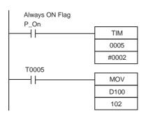
TIM0005 is started when the power is turned ON. After 0.2 s (200 ms) elapses, the TIM0005 contact turns ON and the data stored in D100 will be moved to CIO 102 as the conversion data for analog output 1.
