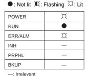
There may be a CPU error or a fatal error if operation stops (i.e., the RUN indicator turns OFF) and the ERR/ALM indicator lights.
