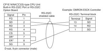
\* DR and ER signals are not supported by the N□□S(1)-type CPU Unit.
