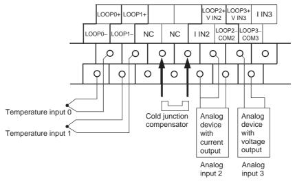
Wiring for Analog Inputs
