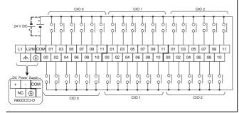
**Input Wiring Diagram**
