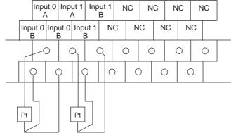
Temperature input 0 Temperature input 1
