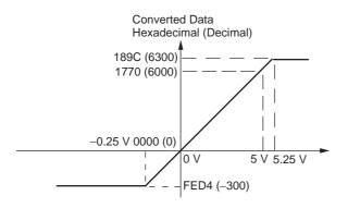
Voltages in the 0 to 5 V range correspond to hexadecimal values 0000 to 1770 (0 to 6,000). The range of data that can be converted is FED4 to 189C hex (-300 to 6,300).
