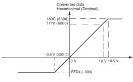
When the resolution is 1/6,000, the 0 to 10 V range correspond to hexadecimal values 0000 to 1770 (0 to 6,000). The range of data that can be converted is FED4 to 189C hex (-300 to 6,300). A negative voltage is expressed as a two's complement.
