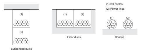
When wiring in the same duct, use shielded cables and connect the shields to the GR terminal to reduce noise.
