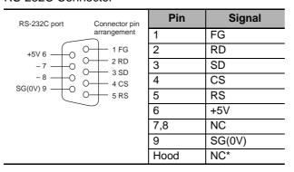
\* The hood and the connector hood to which it is connected will have the same electrical potential.
