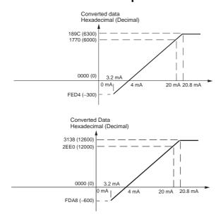
When the resolution is 1/6,000, the 4 to 20 mA range correspond to hexadecimal values 0000 to 1770 (0 to 6,000). The range of data that can be converted is FED4 to 189C hex (-300 to 6,300). Current in the range of 3.2 to 4 mA is expressed as a two's complement.
