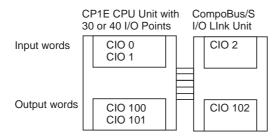
The input word (m+1) contains the data from the Master Unit and the CompoBus/S communications status.
