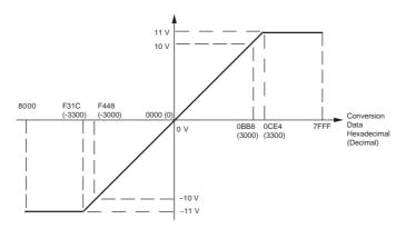
When the resolution is 1/12,000, the hexadecimal values E890 to 1770 (-6000 to 6000) correspond to an analog voltage range of -10 to 10 V.
