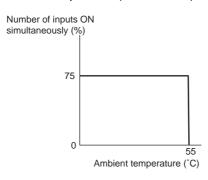
According to the ambient temperature, there are restrictions on power supply voltage and output load current for the CPU Units connected with the Expansion I/O Units (CP1W-8ER/16ER/20EDR1/32ER/40EDR). Use the PLC in the range of the power supply voltage and output load current as show below.
