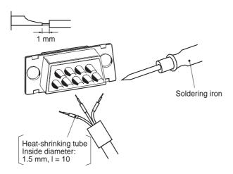
Return the heat-shrinking tube to the soldered portion, then heat the tube to shrink it in place.
