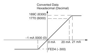
Currents in the 0 to 20 mA range correspond to hexadecimal values 0000 to 1770 (0 to 6,000). The range of data that can be converted is FED4 to 189C hex (-300 to 6,300). A negative current is expressed as a two's complement.
