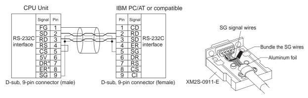
$^*$  DR and ER signals are not supported by the NDDS(1)-type CPU Unit.
