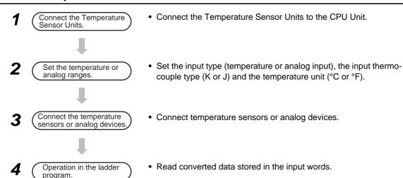
1 Connect the Temperature Sensor Unit to the CPU Unit.
