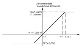
When the resolution is 1/6,000, the 0 to 5 V range correspond to hexadecimal values 0000 to 1770 (0 to 6,000). The range of data that can be converted is FED4 to 189C hex (-300 to 6,300). A negative voltage is expressed as a two's complement.
