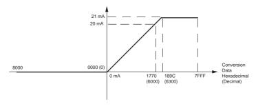
When the resolution is 1/12,000, the hexadecimal values 0000 to 2EE0 (0 to 12000) correspond to an analog voltage range of 0 to 20 mA.
