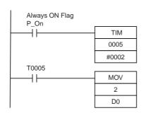
TIM0005 is started when the power is turned ON. After 0.2 s (200 ms) elapses, the TIM0005 contact turns ON and the analog input 1 conversion data stored in CIO 2 is transferred to D0.
