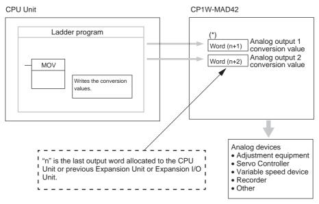
\* Words (n+1, n+2) can be used for either the set data or the analog output conversion value.
