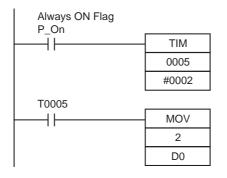
TIM0005 is started when the power is turned ON. After 0.2 s (200 ms) elapses, the TIM0005 contact turns ON and the converted data from analog input 0 that is stored in CIO 2 will be transferred to D0.
