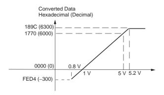
Voltages in the 1 to 5 V range correspond to hexadecimal values 0000 to 1770 (0 to 6,000). The range of data that can be converted is FED4 to 189C hex (-300 to 6,300).
