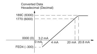
Currents in the 4 to 20 mA range correspond to hexadecimal values 0000 to 1770 (0 to 6,000). The range of data that can be converted is FED4 to 189C hex (-300 to 6,300). Current in the range of 3.2 to 4 mA is expressed as a two's complement. If an input is below the range (i.e., less than 3.2 mA), the open-circuit detection function is activated and the data becomes 8,000.
