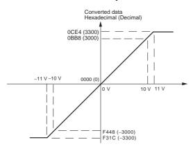
When the resolution is 1/6,000, the -10 to 10 V range correspond to hexadecimal values F448 to 0BB8 (-3,000 to 3,000). The range of data that can be converted is F31C to 0CE4 hex (-3,300 to 3,300). A negative voltage is expressed as a two's complement.
