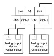
Note 1 Use 2-conductor shielded twisted-pair cable for the I/O wiring, and do not connect the shield AG terminal.
