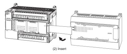
Attach the cover to the CPU Unit's or the Expansion I/O Unit's expansion connector.
