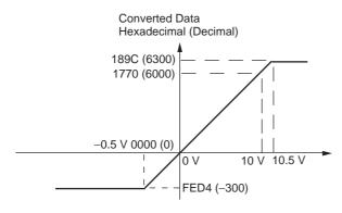
Voltages in the 0 to 10 V range correspond to hexadecimal values 0000 to 1770 (0 to 6,000). The range of data that can be converted is FED4 to 189C hex (-300 to 6,300).
