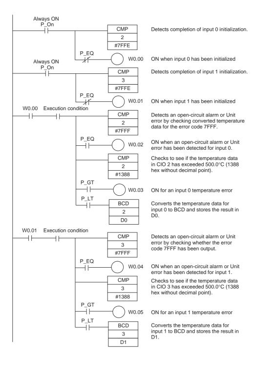
(b) The following programming example shows how to convert the data for temperature input 0 to BCD and store the result in D0 and D1. "#0001" is stored in D1 when the input data is a negative value. The following system configuration is used.
