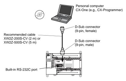
Connect the CX-Programmer to the built-in RS-232C port by XW2Z-200S-CV/500S-CV RS-232C cable.
