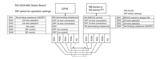
Note Do not use NS-AL002, when connecting the built-in RS-422A port of the NB-series PT.
