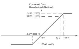
When the resolution is 1/12,000, the 0 to 10 V range correspond to hexadecimal values 0000 to 2EE0 (0 to 12,000). The entire data range is FDA8 to 3138 hex (-600 to 12,600). A negative voltage is expressed as a two's complement.
