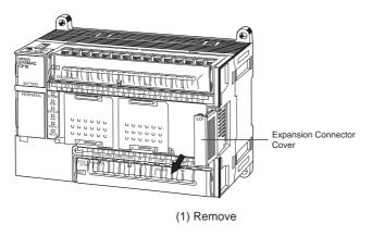
Insert the Expansion I/O Unit's connecting cable into the CPU Unit's or the Expansion I/O Unit's expansion connector.
