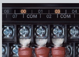
Input/output terminal LED indicators for quick troubleshooting
