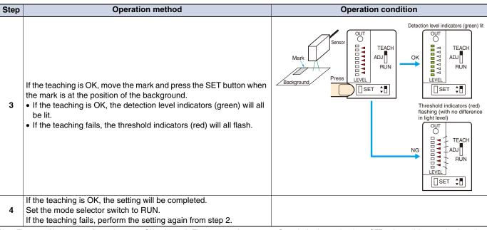
Note: These teaching steps are for turning output ON at the mark. The output can be set to turn On at the background and turn OFF at the mark by reversing the order of teaching.
