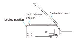
Note:1.To maintain the fiber characteristics, make sure that the lock is released before removing the fibers.
