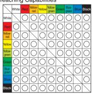
\* The above chart shows the combinations of colors for which teaching is possible at a sensing distance of 12 mm.
