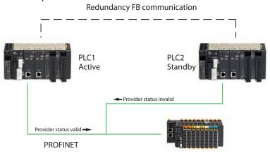
The preferred solution for the Redundancy FB communication is EtherNet/ IP. This is because it is easy to set up datalinks to transfer data independent of the PLC program. It is also fast, reliable and easy to install. It can run on the same network as the PROFINET communication, but to have higher reliability we recommend it is used over a seperate (ethernet) network.
