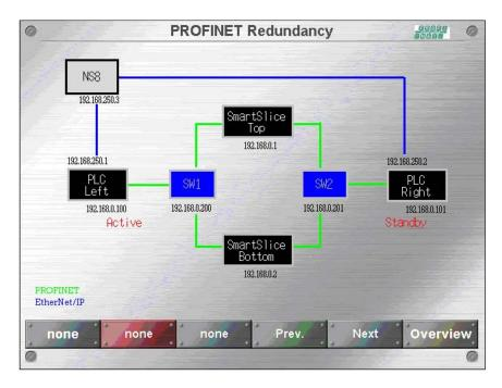
For each of the devices the IP-addresses are shown. These IP-addresses can be used to communicate to each of the devices.
