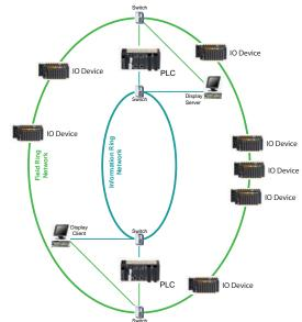
For the implementation of the redundancy functionblock this network setupis used. There is a Fieldnetwork or Controlnet and a Informationnetwork or Infonet.
