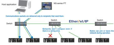
Star topology using Ethernet switch technology
