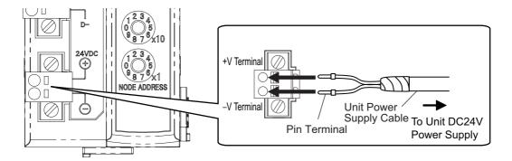
Mount a pin terminal, or equivalent to the unit power supply cable so that it will not be displaced. Do not wire a power supply to the communications path of the Distributed Sensor Units. The Units may be damaged.
