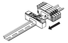
4 Use the DIN Track End Plates (PFP-M) that are provided to remove any gaps between the Units and secure them in place. Replace the protective cap that you removed in step 3 to the Sensor Amplifier on the right end.
