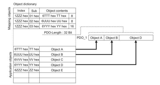
The figure below shows an example of PDO mapping.
