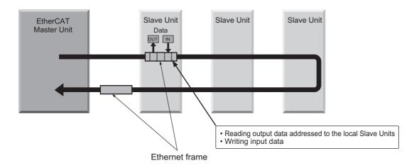
It is the "EtherCAT telegram" stored directly in an Ethernet frame that exchanges data regularly between the EtherCAT Master Unit and Slave Units.
