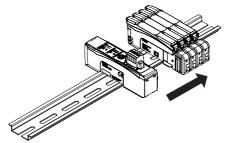
2 Keep the Distributed Sensor Unit pressed against the DIN Track as you lift it up, and then
