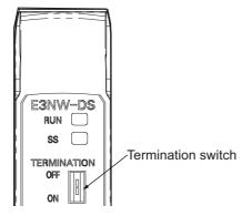
As shown in the following diagram, turn ON the DS-Bus termination switch only on the last Distributed Sensor Unit on the DS-Bus network. Turn it OFF on all other Distributed Sensor Units.
