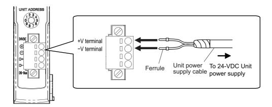
Attach ferrules to the Unit power supply cable wires and connect them securely so that they do not come loose.
