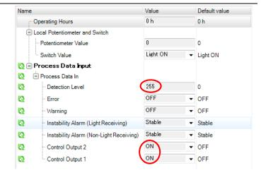
25 In the PLC Memory Window of CX-Programmer, check that the value of D10104 is as shown below. D10104
