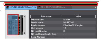
2 Right-click the device icon of EtherNet/IP Coupler Unit (Unit 0) and select Coupler Connection (USB) - Transfer to Coupler from the menu.
