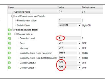
22 In the PLC Memory Window of CX-Programmer, check that the value of D10104 is as shown below.
