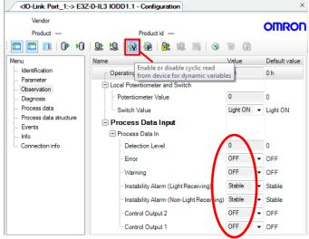
Check that Operation mode switch on Photoelectric Sensor is set to Light ON (factory setting).
