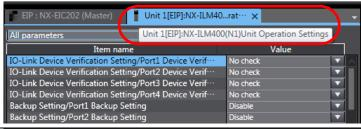
3 Select **▼Port1 - Port1 IO-Link Device Configuration Data**from the pull-down list (just above the column "Item name") to narrow down the parameters.
