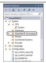
6 Checking that EtherNet/IP is operating
