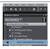
In the TCP/IP Settings view of the Built-in EtherNet/IP Port Settings tab page, set the IP Address\*1 to enable connection to the PMAC.
