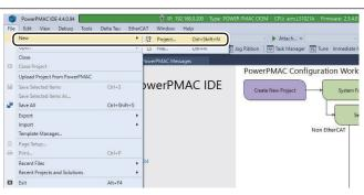
Enter the type of project for which EtherNet/IP can be set, desired project name, and the save destination, and click the OK button.
