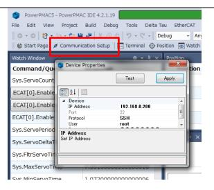
In the Device Properties dialog box, select *No Device* for IP Address, then click the **Apply** button.
