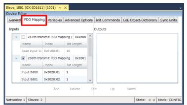
Check Inputs to make sure that only the 258th transmit PDO Mapping 0x1B01 check box is selected.
