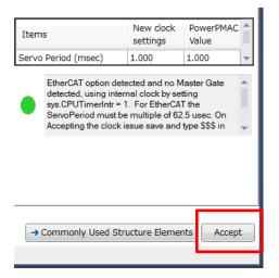
If you have changed the servo frequency setting, type the save command in the Terminal tab page of Power PMAC IDE.
