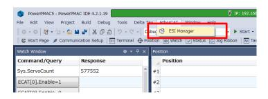
2 Confirm that Omron GX-Digital IO.xml is registered in the ESI file list of ESI Manager.
