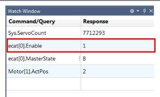
After making sure that correct communications are available, run the ECAT[0].Enable=0 command from the Terminal tab page to stop EtherCAT communications.
