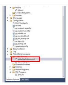
In the programming area of the global definitions.pmh tab page, write the set values to be set automatically upon power-on.
