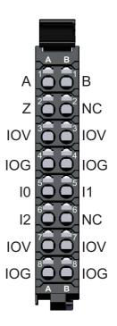
Note The encoder power supply output (24 V and 0 V) is provided power from the I/O power supply connected to the Communications Coupler Unit or an Additional I/O Power Supply Unit.
