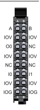
Note The sensor power supply output (24 V and 0 V) is provided power from the I/O power supply connected to the Communications Coupler Unit or an Additional I/O Power Supply Unit.
