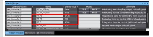
You can use the feature of changing current values on the ST Editor to change and monitor the current values of variables and perform autotuning as well. For details, 7-2 Operations Used for Both Online and Offline Debugging described in the Sysmac Studio Version 1 Operation Manual (W504).
