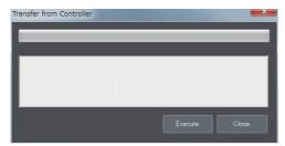
If this command is executed when a project is already open, the project settings are overwritten with the GEM setting data transferred from the Controller.
