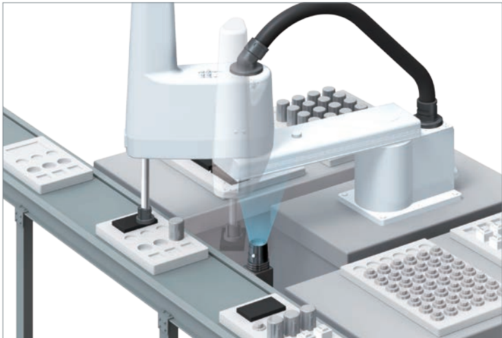
Pick & Place with position correction
