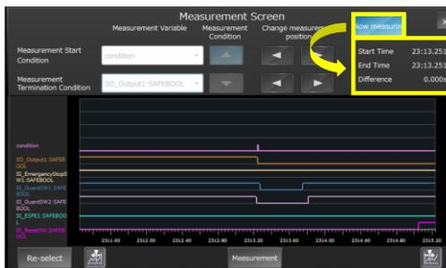
5. Press the [◀] or [▶] button to change the object to measure. You can find the next (or previous) data that satisfies the measurement conditions.
