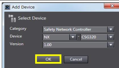
5. The controller is added. Implement necessary settings.
