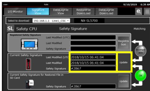
A signature for a restored file in the SD card is read out when a page is opened or the [Update] button is pressed.
