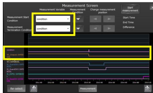
3. Set the measuring conditions for the selected variable, Rising or Falling.
