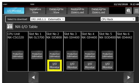
4. The status of the selected I/O unit is indicated. Press the [◀] or [▶] buttons to see other I/O units. The display is automatically updated at 1 second interval.
