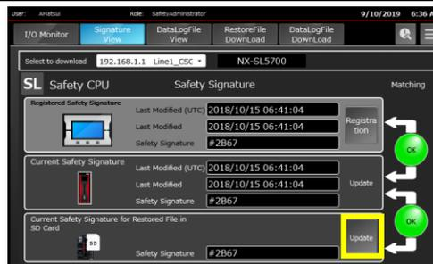
4. The current safety signature of the restored file in the SD card is read out. Check if the safety signature is the same as the current safety signature. If they are the same, the [OK] lamp on the right turns green.
