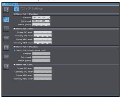
3 Click the FINS Settings Button and set the network address for Ethernet port 1. Set the routing table as required.
