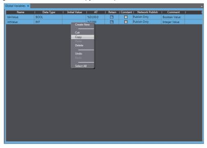
Paste the device variables in a spreadsheet, delete unnecessary rows, and sort and copy the remaining rows. Refer to A-1 Clipboard Format for Device Variable Table Data on page A-2 for information on the order of the rows.
