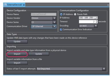
The global variables of the CJ-series PLC are transferred and registered as device variables.
