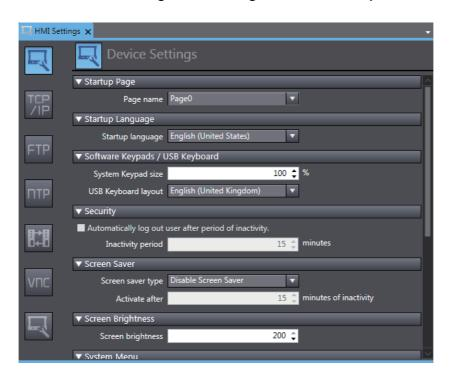
Click the TCP/IP Settings Button and set the IP address for Ethernet port 1 in the TCP/IP Settings. Also set the subnet mask and default gateway as required.
