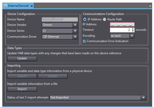
Make the following settings for the external connected device.
