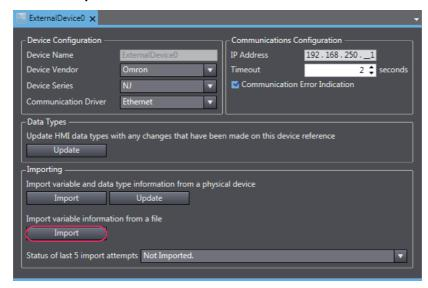
The variables are copied to the device variable table of the HMI project.
