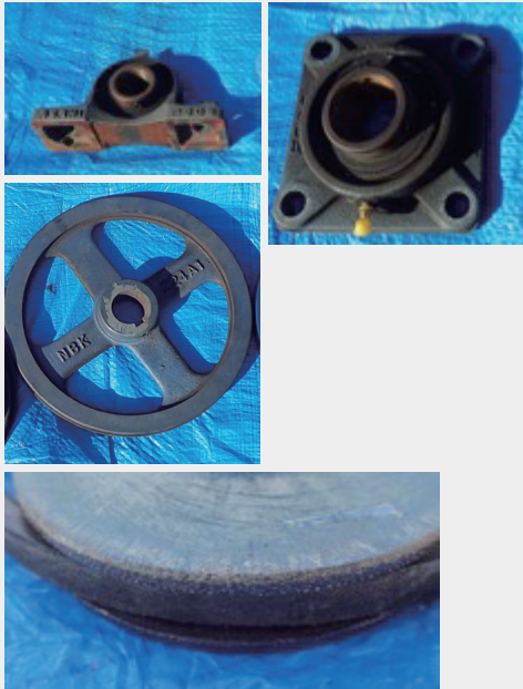
Belt and pulley worn down by friction
