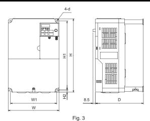
Dimensions in mm (inches)/Mass in kg (lb)/Heat Loss (W)
