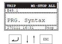
Press the ∠ key to show the information on the past trips (six trip errors) recorded in the Inverter and the information on the warning (one warning).
