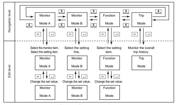
In addition to the above, the LCD Digital Operator has the following three called modes. At any of the above levels and in any operating state, you can call these modes by pressing the key(s) shown to the right of the down arrow above each screen, as shown on the next page. After calling these screens, you can press the ESC key to restore the operating state before the call.
