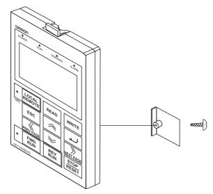
4 Remove the old battery using a thin slotted screwdriver.
