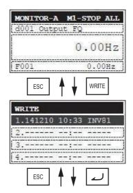
When no Inverter parameter setting data is stored in the LCD Digital Operator, "--" is shown.
