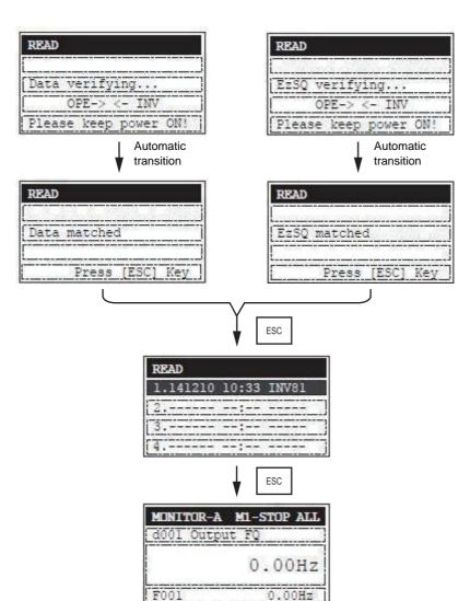
When the verification of the parameter setting data or DriveProgramming program is completed, the result appears.
