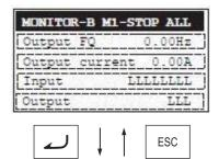
Press the we key to show the cursor in the first parameter line of the "d" group monitor function.
