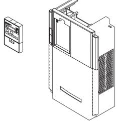
2 Install the LCD Digital Operator on the Inverter.
