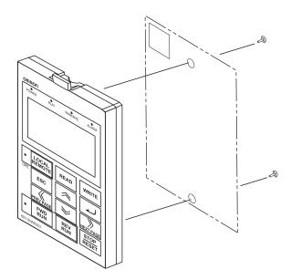
**Remove the Digital Operator and** the operator connector from the Inverter.
