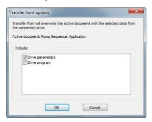
After pressing ok, the parameters will start to be transferred:
