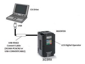
**3.** Use the CX-Drive autodetect hunction in order to go online with the 3G3RX inverter:
