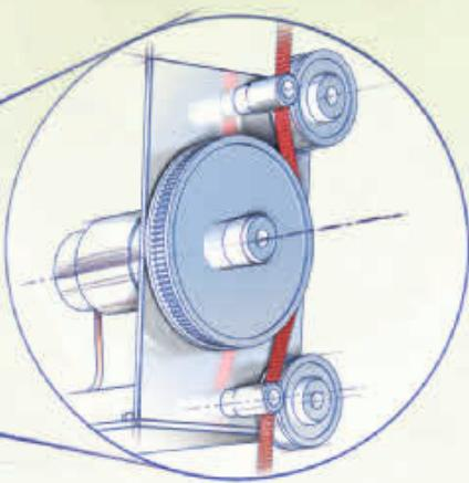
» The second encoder for position feedback avoids errors due to motor sheave slipping and rope extension
