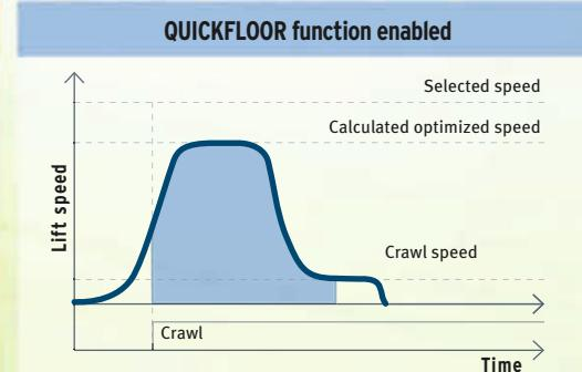
One optimized speed is selected ensuring lift comfort is maintained and crawl time is minimized
