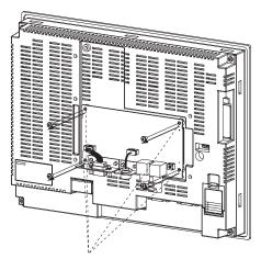
Remove the screws securing the four corners.
