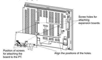
(2) Push firmly on the connector end of the board and make sure that it is inserted sufficiently.
