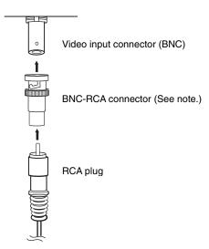
\* The BNC-RCA connector is not provided with the RGB and Video Input Unit (NS-CA002).
