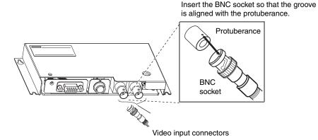
(2) After inserting the BNC socket, twist it clockwise until it locks into place.
