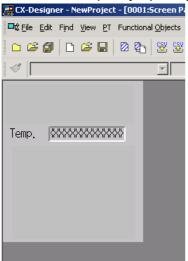
2. Double-click the object to display the Properties Dialog Box. Select the *Temporary input* option under *Function* on the General Tab Page.
