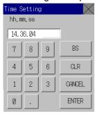
The date is entered in the yyyy.mm.dd format and the time is entered in the hh.mm.ss format.
