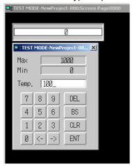
When the focus is on the numeral display and input object, the input value is displayed in the temporary input object. Click the **Command** Button to overwrite the present values with the new input value.
