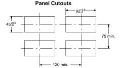
The values given above are recommended values. Do not gang-mount with dimensions less than these recommended values.
