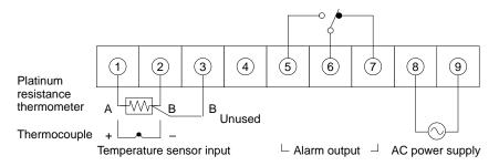
**Note:** Terminals 5, 6, and 7 are not used by models with no alarm output. (These terminals are open only for models incorporating the display function.)
