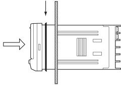
Fit the adaptor into the grooves on the left and right sides of the rear case, then push it until it contacts the panel to secure the K3MA-L.
