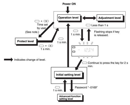
$\textbf{Note:} \ \ \textbf{The move-to-protect-level time can be set in the advanced-function setting level}.$
