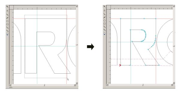
If the object selection method is set to "Include" a portion of the text "O" gets included when the text "R" is selected. Click the object while holding down the [Ctrl] key and delete the points for the text "O."
