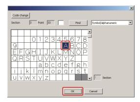
Glyph "A" of "LM\_Font.osf" will be replaced by the text image drawn, and will be saved.
