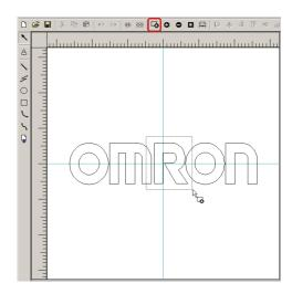
2 Click [View] on the menu bar, select [Guide line] to display horizontal and vertical lines, and place them on the edit positions.
