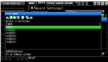
Use the  $\nabla\triangle$  key to move the cursor to the created "TEST" folder, and press the ENTER key.
