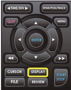
This key is used to switch the window mode.
