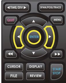
Press the ◀, ▶, and ENTER keys at the same time to display the password setting screen shown below. Specify a 4 digit password.
