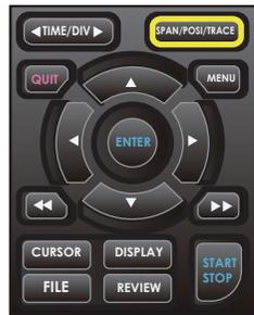
Switches the display in the digital display.
