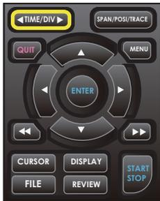
Press the left/right key of the TIME/DIV key to change the time axis display width.
