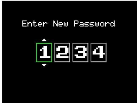
Use the ◀, ▶, △, ▽ keys to select numbers. Press the ENTER key to confirm the password.
