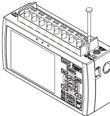
**4** Connect the DC cable to the DC power supply.
