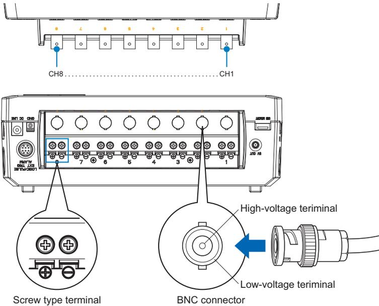
The screw type terminal and the BNC connector are internally connected. Data entered to either of them can be measured.
