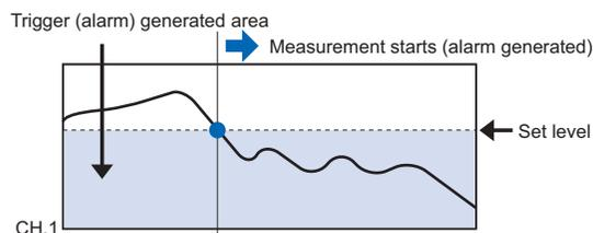
**Win In** : Used to specify the upper and lower limits for each channel. When the signal level goes within (or is within) either limit, a trigger/alarm is generated.
