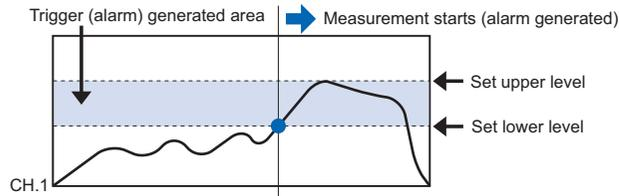
Win Out:Used to specify the upper and lower limits for each channel. When the signal level goes outside (or is outside) either limit, a trigger/alarm is generated.
