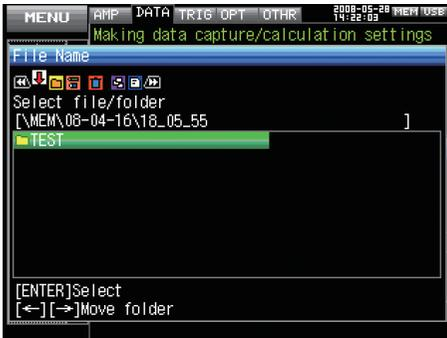
Use the  $\nabla/\Delta$  key to move the cursor to the created "TEST" folder, and press the ENTER key.
