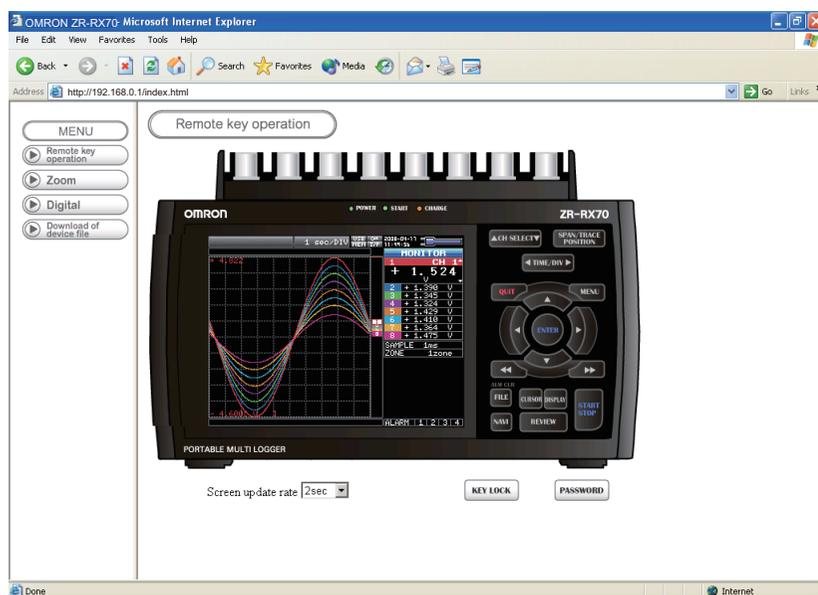
Remote key operation..... Allows ZR-RX70 operation.
