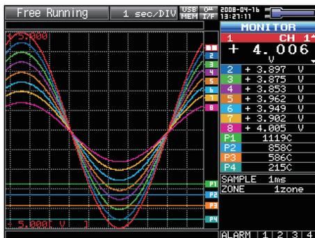
When in Free Running status, you primarily set up the system to capture data. You can check the current input signal as a waveform or digital values.
