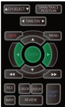
Press the ◀, ▶, and ENTER keys at the same time to display the password setting screen shown below. Specify a 4 digit password.
