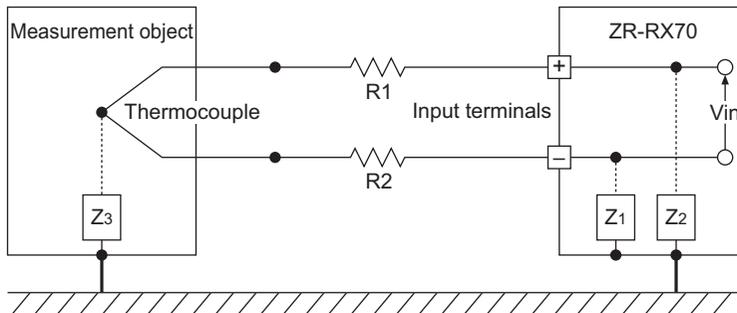
**Connect the signal chassis GND and the measurement device chassis ground.**
