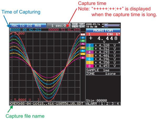
During data capture, data is captured into the Internal memory or USB device.
