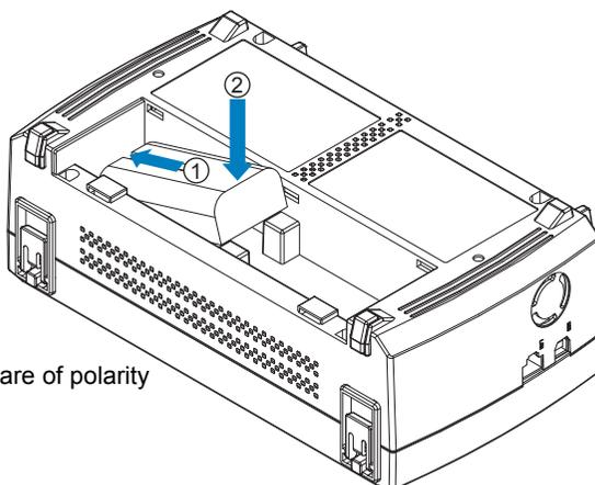
Attach the battery with care of polarity and insertion direction.
