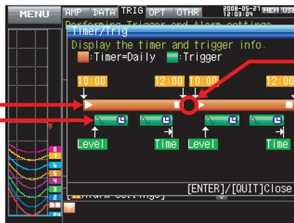
A trigger generated in this interval will not start data capture.
