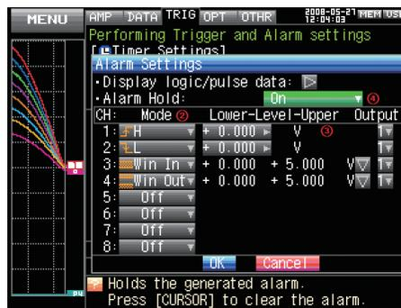
Holds the generated alarm. Press [CURSOR] to clear the alarm.
