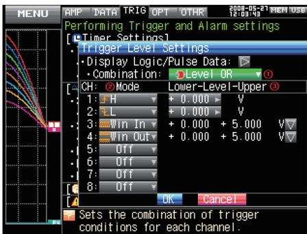
Sets the combination of trigger conditions for each channel.
