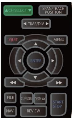
Press this switch to select the channel to change the settings in the Waveform + Digital or X-Y screen.
