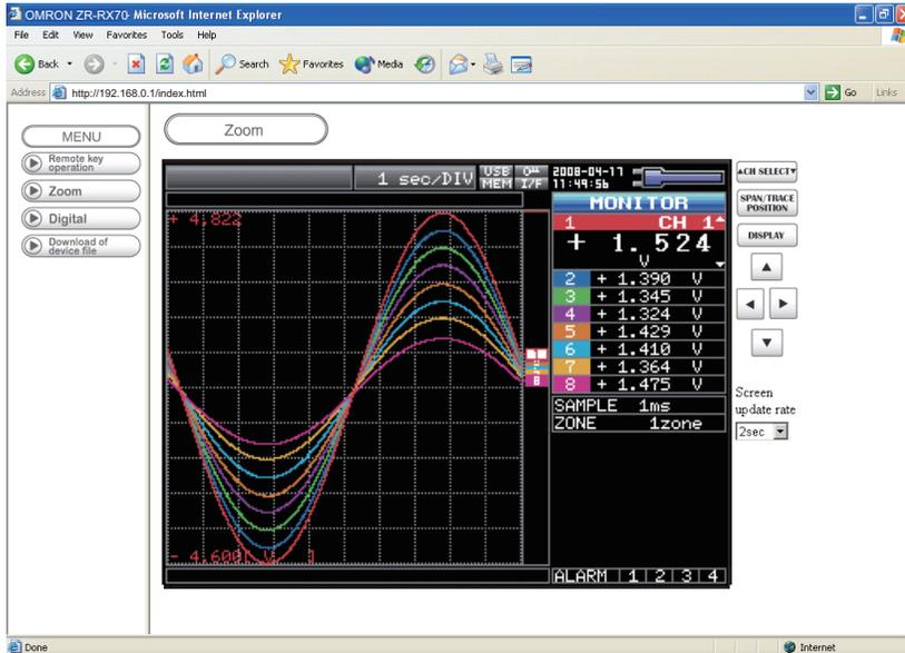
CH SELECT ..... Press this switch to move the active channel in the Waveform + Digital or X-Y screen.
