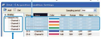
Channels 1 to 4 on ZR-RX70 grouped by "Voltage" and "Sampling Period (1ms)"
