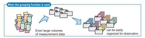
The "grouping" function is for performing observation with multiple channels set as a single group.
