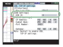
The USB ID and the IP address can be set in the following window.
