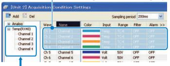
Channels 1 to 4 on ZR-RX40 grouped by "Temperature" and "Sampling Period (200ms)"
