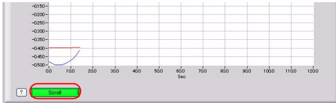
The scrolling operation will be halted, enabling past data to be displayed in the scroll bar. Moreover, moving the cursors enables the cursor level values to be viewed. To return to the waveform scrolling operation, click the [Scroll] button once again.
