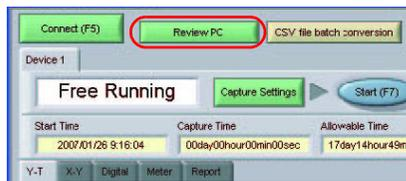
The file selection screen opens. Open the file to which the data was captured. A thumbnail waveform is displayed at the left of each file name, enabling you to confirm the data contents without opening each file.
